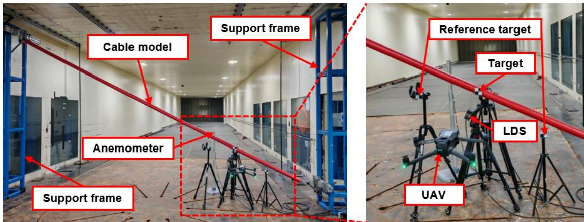
Figure 1. Wind tunnel experimental setup for vortex-induced vibration of the stay cable.
