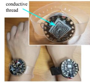
Fig. 2. TouchSync Prototypes.
