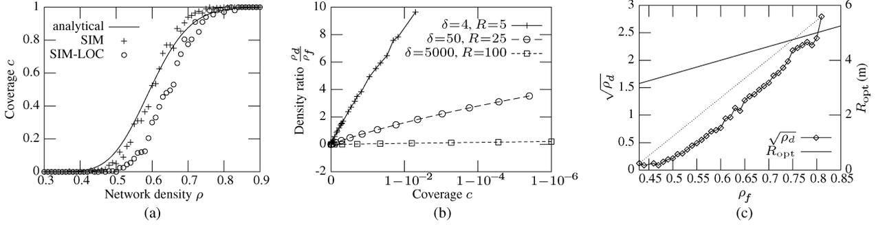
Fig. 6. Simulation results of random networks. (a) Coverage versus network density ( $\delta = 4$ ,  $R = 5$  m). (b) Density ratio  $\rho_d/\rho_f$  versus coverage in  $\log_{10}$  scale with various PSNRs. (c)  $\sqrt{\rho_d}$  versus  $\rho_f$  with optimal fusion range  $R_{\text{opt}}$  ( $\delta = 4$ ).
