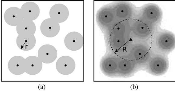
Fig. 2. (a) Coverage under the disc model, where  $r = 17$  m that is computed by (2). (b) Coverage under the fusion model, where grayscale represents  $P_D$ .
