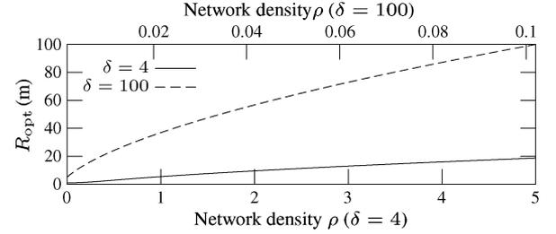
Fig. 4. Optimal fusion range versus density ( $\alpha = 5\%$ ,  $\beta = 95\%$ ).
