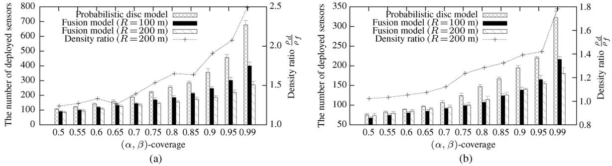
Fig. 5. Number of deployed sensors versus achieved  $(\alpha, \beta)$ -coverage. (a) Random networks. (b) Regular networks.
