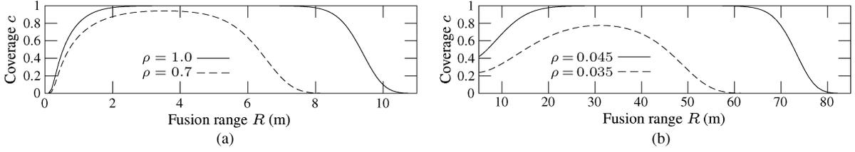
Fig. 3. Coverage versus fusion range ( $\alpha = 5\%$ ,  $\beta = 95\%$ ). (a)  $\delta = 4$ . (b)  $\delta = 100$ .
