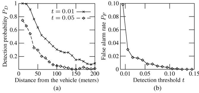
Fig. 1. Sensing performance of an acoustic sensor in detecting vehicle. (a) Detection probability versus the distance from the vehicle. (b) False alarm rate versus detection threshold.
