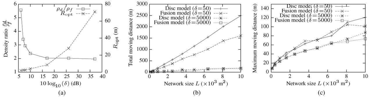
Fig. 7. Simulation results of regular and mobile networks. (a) Density ratio of regular networks versus PSNR with optimal fusion range. (b) Total moving distance of mobile sensors versus network size. (c) Maximum moving distance of mobile sensors versus network size.
