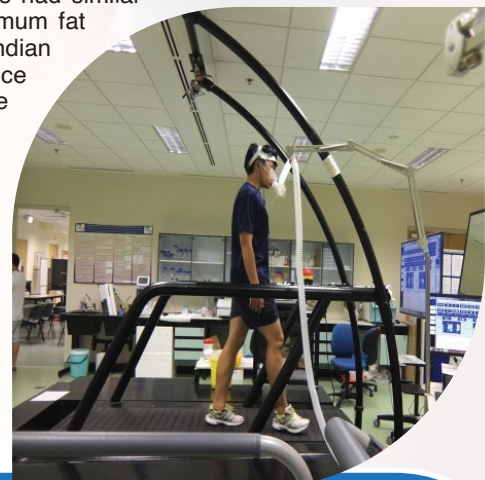
Figure 2. Measuring expired gases into a metabolic cart during exercise. A tube and mouthpiece were fixed via a headpiece onto the participant and expired air was collected into a metabolic cart for analysis.
