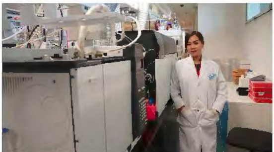
Complete set-up of GC/LC-ICP-QQQ for speciation studies.
