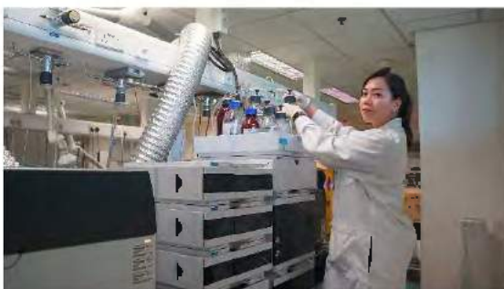
Changing LC mobile phase for LC-ICP-MS arsenic speciation.
