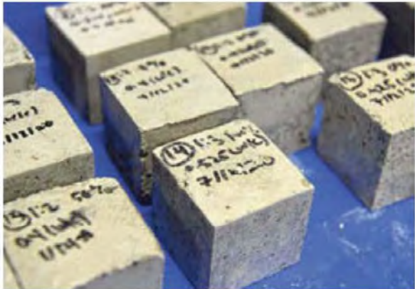
Samples of sustainable construction materials made from waste residue. Nanyang Technological University’s project was one of 12 awarded a combined $55 million in grants under the national Low-Carbon Energy Research Funding Initiative, which seeks to reduce carbon dioxide emissions.
