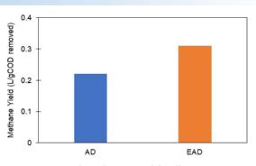
COD removal efficiency and methane yields were 20-40% higher in a EAD system.
