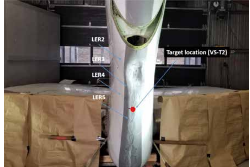
Vertical stabilizer setup (VS-T2)
