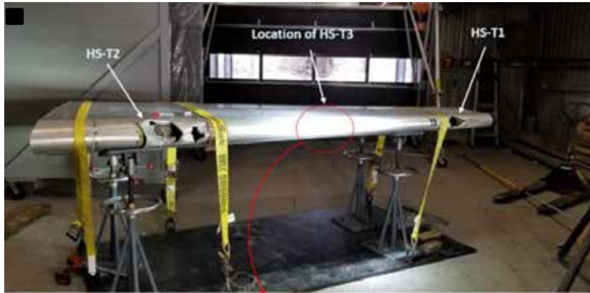
Horizontal stabilizer setup (HS-T3)
