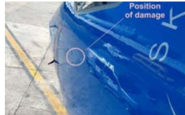
737 was hit by a drone during the landing process (17 th Nov. 2017 )
