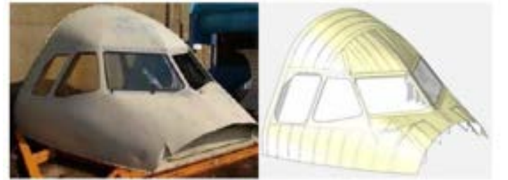
Figure 1: Airliner cockpit for impact testing (left) and computer reference model
