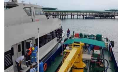
Bunkering operation conducted at sea (ship to ship)
