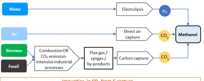
**Direct hydrogenation** of *pure* CO<sub>2</sub> and H<sub>2</sub> simplifies MeOH synthesis chemistry. Fewer reactions and by-products
