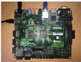
The RISC-V based platform is implemented on the Xilinx Zynq-7000 FPGA device.
