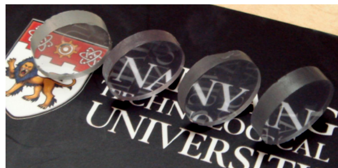
The photos of transparent ceramics (from left to right: YAG, Nd:YAG, Y 2 O 3 , Nd:Y 2 O 3 )
