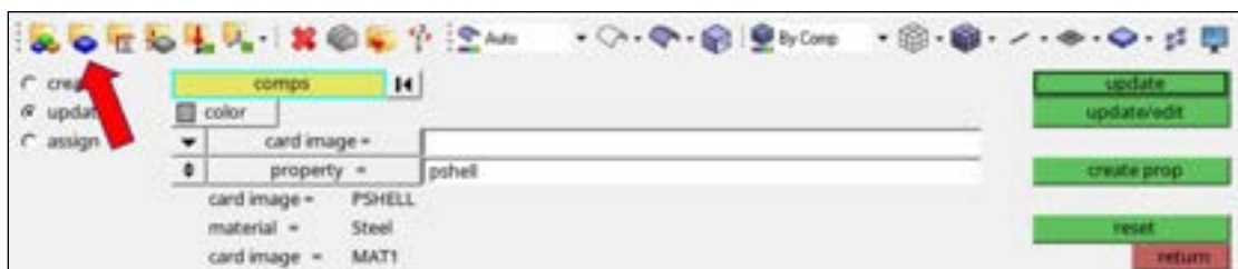
Figure 4.9: Assign materials and properties to components
