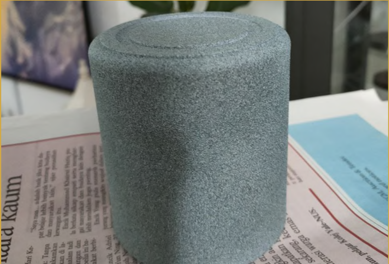
Testing the stone finish on the TERRAPIN bottle for enhanced grip even when wet.
