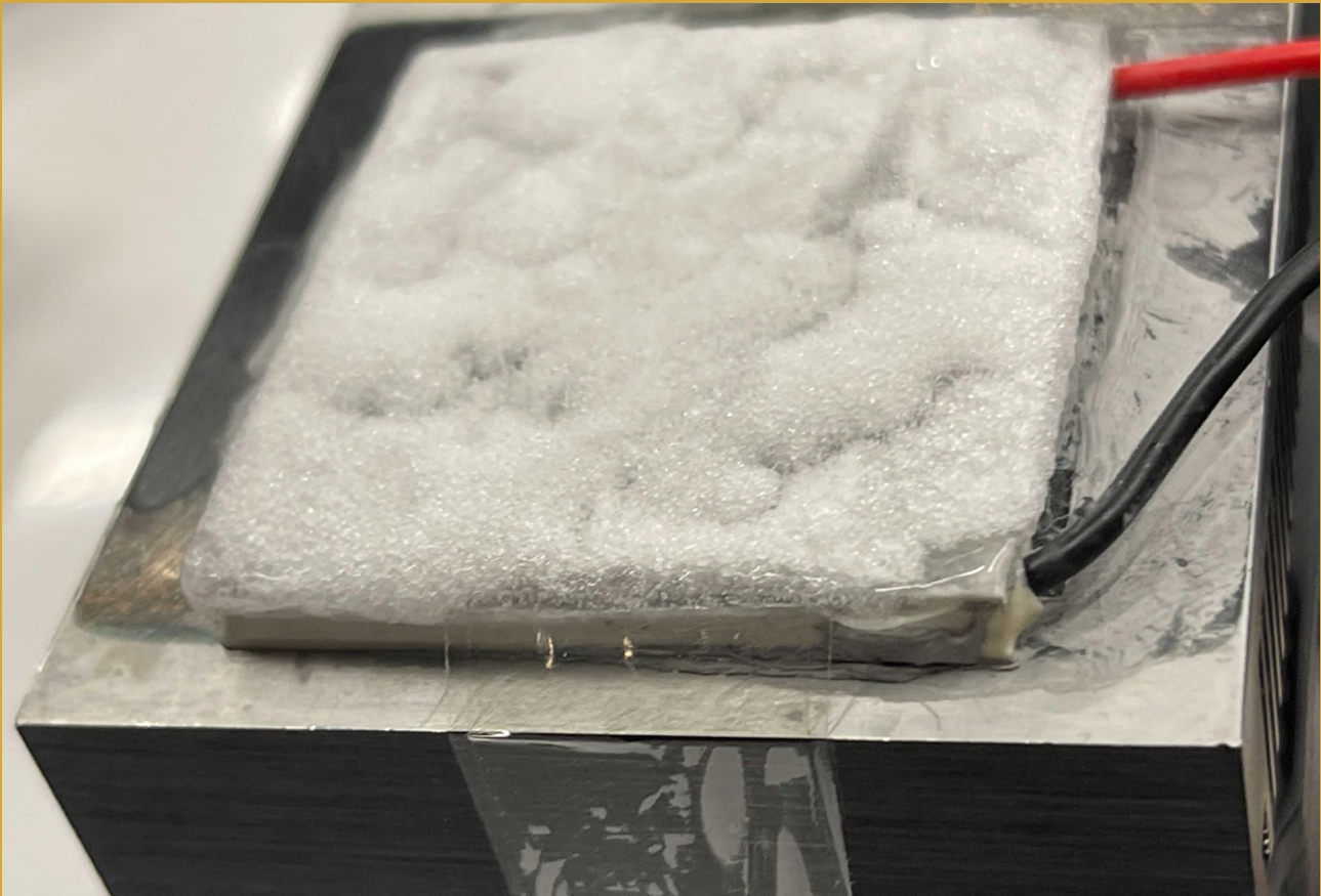
Our testing of the thermoelectric cooler - fan cooling system , capable of reaching -10^{\circ}\text{C} .
