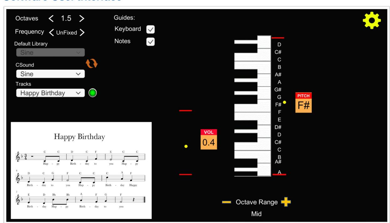
The yellow dots on the screen represent the current position of the user's hand detected by the Leap Motion. Users can customise the software by setting the number of octaves, display guides, sine wave function and background tracks.
