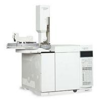
GC-FID is used in analytic chemistry for separating and analyzing compounds that can be vaporized without decomposition. The GC- FID can detect almost all carbon containing compounds.
