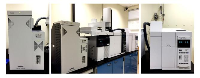
Besides the liquid sampling, this GCMS system also allows sampling of gas and slurry samples. Air or gas samples can be collected into a sorbent packed tube and introduced into the GCMS via Thermal Desorber (Markes TD-100). Headspace (HS) and thermal sorption probe (TSP) sampling are the other alternative methods which available on this system.
