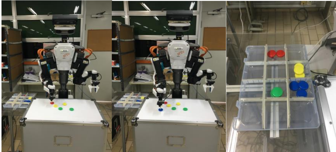
Figure 2: Sorting out of small parts based on the color features with a dual-arm
