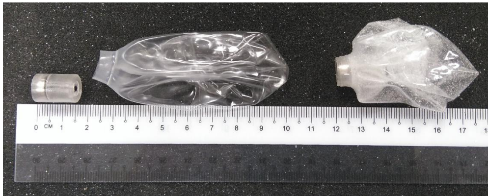
Figure 2: Inner capsule, outer balloon and the assembled IGB device (left to right).
