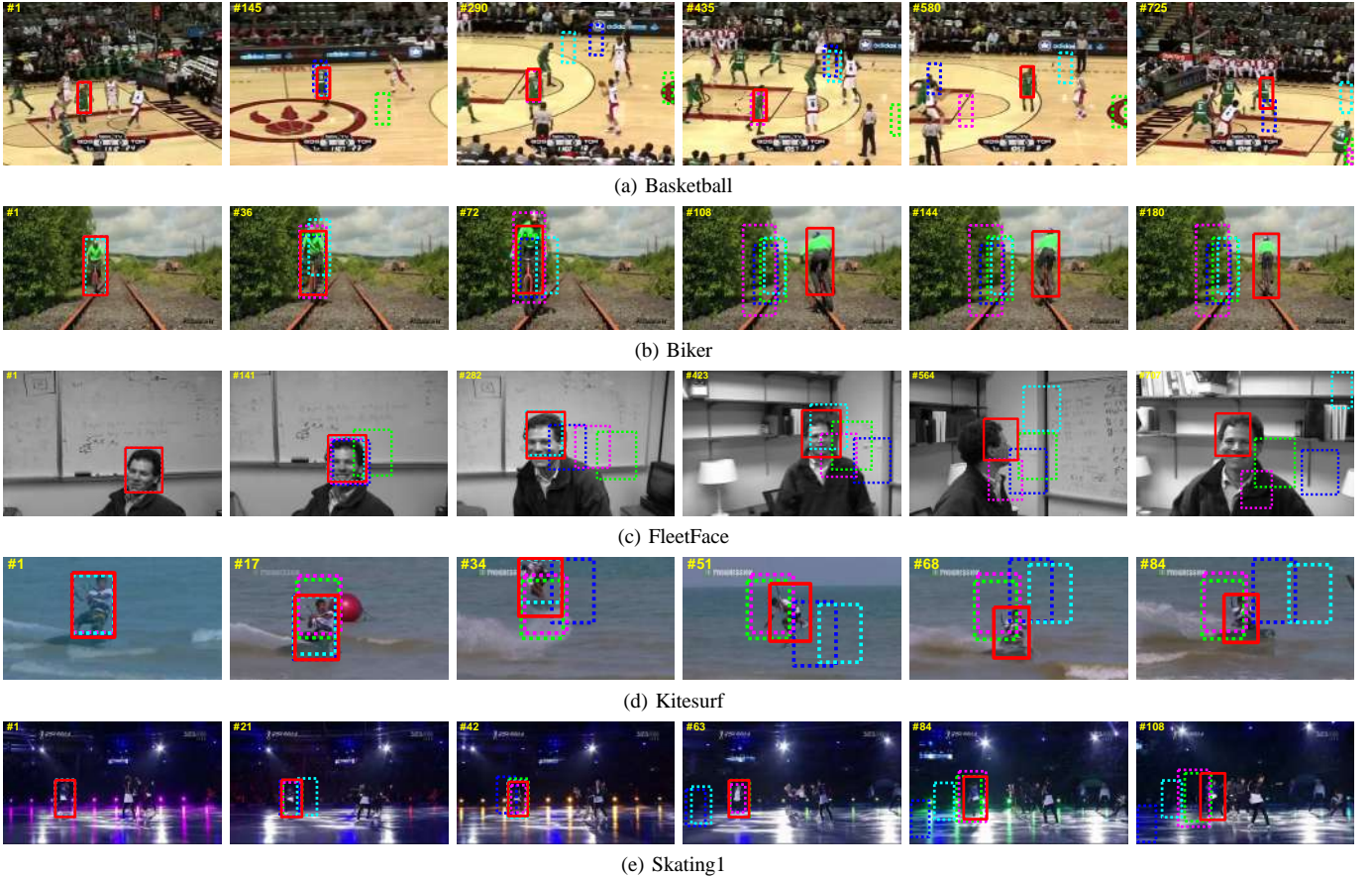
Fig. 3: Qualitative results on sequences with non-rigid object deformation. The purple, green, cyan, blue and red bounding boxes refer to ASLA[33]_RAW, ASLA[33]_HOG, l_1 _APG [60], CT_DIF [37] and our tracker respectively. This figure is better viewed in color.
