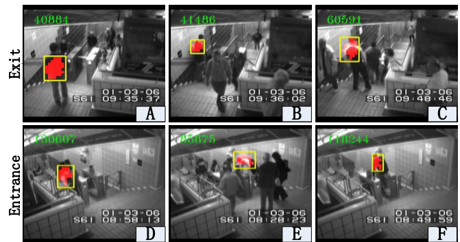
Figure 7. Examples of local abnormal events detection for Subway dataset. The top row and bottom row are from exit and entrance video sets, respectively, and red masks in the yellow rectangle indicate where the abnormality is, including wrong directions (A-D) and no-payments (E-F).
