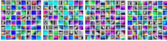
Fig. 5. Visualization of the learned convolution filters for the first layer of CNN-CS, CNN-TCS, CNN-GS and CNN-HS respectively. They are trained on the Barcelona datasets. Note the visual difference among the learned filters of different CNN-M. The figure is best viewed in color.
