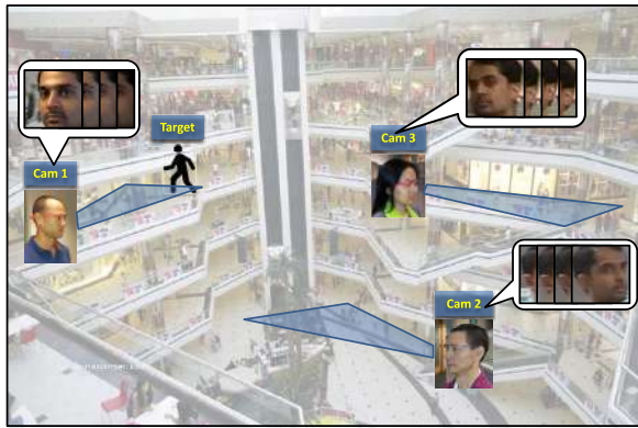
Fig. 1. Illustrative diagram for person re-id using multiple FPV cameras. Three wearable devices (GGs), shown as Cam 1–3, are worn by security personnels at different levels in a multistored congested shopping mall. As a target appears in the field of view (FoV) of a camera (shown using trapezoidal regions on the ground plane), uncluttered face shots of the target can be observed and processed for re-id.
