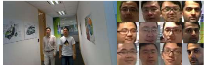
Fig. 10. Database 2 for online re-id. Left: original image captured by GG. Right: four columns show four persons with three images each, captured using three different GGs at different locations/views.
