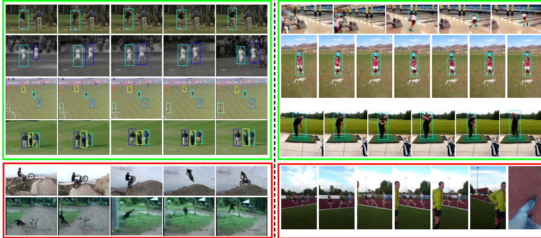
Figure 8. Our action co-localization results on the UCF Sports Plus (left) and SVW Mini (right) datasets. The top rows in the green blocks contain videos with common actions. The bottom rows in the red blocks contain videos that do not have common actions. It can be seen that, the proposed method can handle the cases when there are zero, one or multiple common actions in the videos.
