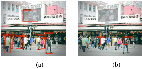
Fig. 4: Example of (a) Person detection by SSD on an input image (b) Suspected object(backpack) detection by SSD on an input image
