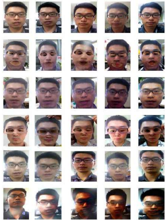
Fig. 5. Examples of Rose-Youtu Liveness Database. From top to bottom: face images in genuine, cropped mask, full mask, upper mask, paper print and video replay versions. (For paper print attack, both warped paper and still paper attacks are considered.) From left to right: face images captured by iPhone 5S, Hasee mobile phone, Huawei mobile phone, iPad and ZTE mobile phone.
