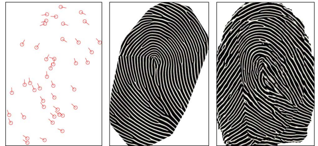
Fig. 12. Different types of new identities that are generated from two different fingerprints. The second row (from left to right): the combined minutiae template, the combined fingerprint from our proposed method (without noising and rendering), and the mixed fingerprint obtained using the approach proposed in [12].
