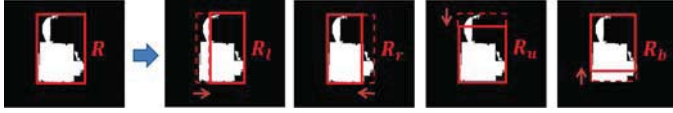
Fig. 3. Shift each side of R into four new bounding boxes ( R_l , R_r , R_u , R_b ) of corresponding sub-segments.
