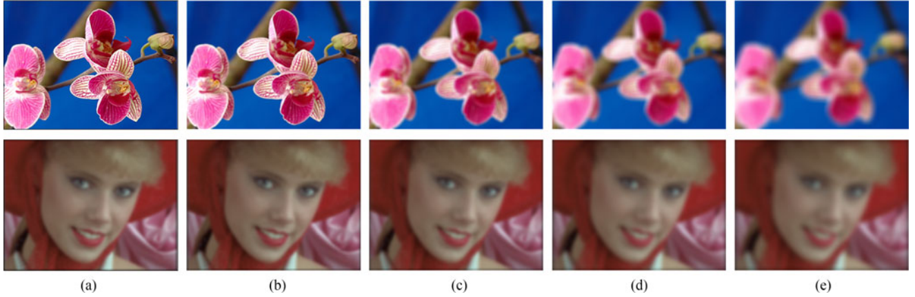
Fig. 2. Scale space representations of two original images. Original image “Orchid” in the first row is of high quality, while the original image “Woman” in the second row is blurred. (a) Original image. (b) Filter size 3 \times 3 , \sigma=2 . (c) Filter size 9 \times 9 , \sigma=4 . (d) Filter size 15 \times 15 , \sigma=6 . (e) Filter size 21 \times 21 , \sigma=8 .
