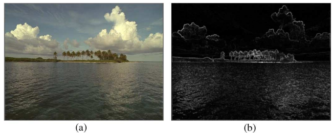
Fig. 2. MLV map. (a) an image (b) MLV map where the brighter pixels show larger MLV than the dark pixels.
