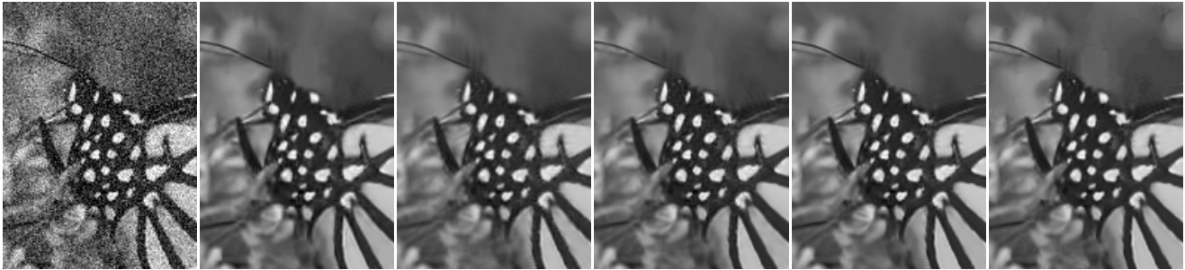
Fig. 2. Denoised fragments of Monarch . From left to right: (a) Noisy image ( \sigma_n = 30 ); (b) BM3D (PSNR = 28.37dB); (c) LPG-PCA (PSNR = 27.79dB); (d) CSR (PSNR = 28.51dB); (e) LASSC (PSNR = 28.27dB); (f) Proposed (PSNR = 28.82dB ).
