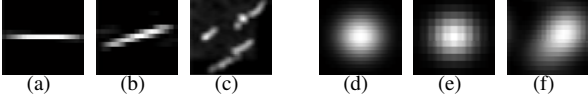
Fig. 2: Examples of blur kernels: (a)-(c) motion blur kernels, (d)-(f) out-of-focus blur kernels.
