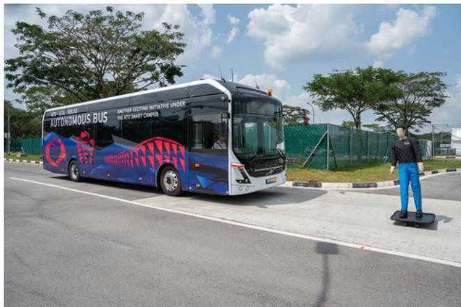
Volvo Buses and Nanyang Technological University (NTU) in Singapore have demonstrated the world's first 12-metre autonomous electric bus. The Volvo bus will soon begin trials on the NTU campus. The 85 passenger Volvo 7900 e-bus is equipped with sensors and navigation controls that are managed by a comprehensive artificial intelligence (AI) system. Ensuring maximum safety and reliability, the AI system is also protected with cyber security measures to prevent unwanted intrusions.
