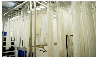
START Centre is a a national-level facility in Singapore to develop and commercialise innovative separation and filtration technologies. This is a membrane production line at START Centre, which produces the tri-bore hollow-fibre membrane ... more
