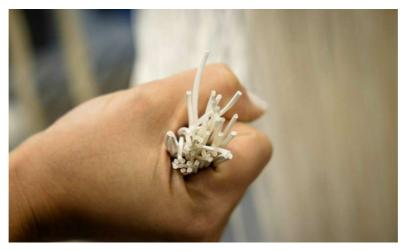
Close up shot of the tri-bore hollow-fibre membrane commercialised jointly by START Centre and Memsift Innovations, which will be used in a new pilot wastewater treatment plant for a semiconductor factory in Singapore. Credit: Nanyang Technological University
