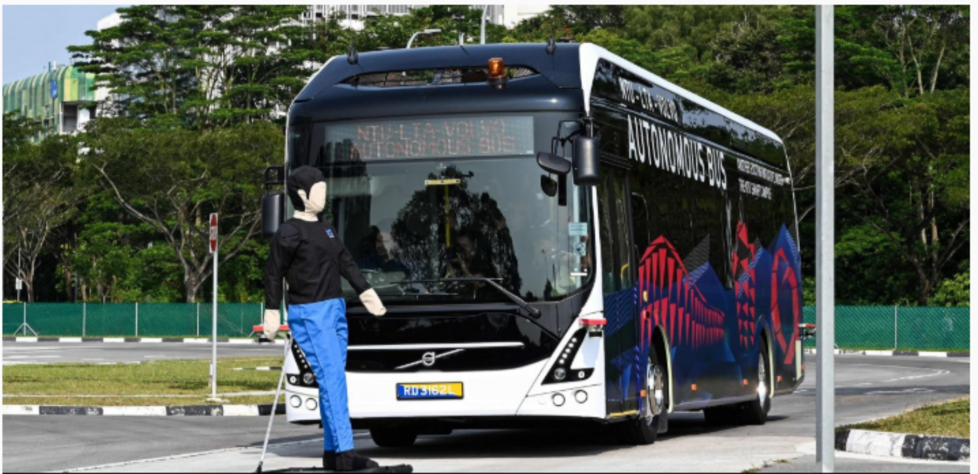
A Volvo AB 7300 electric autonomous bus drives on the track of Centre of Excellence for Testing
