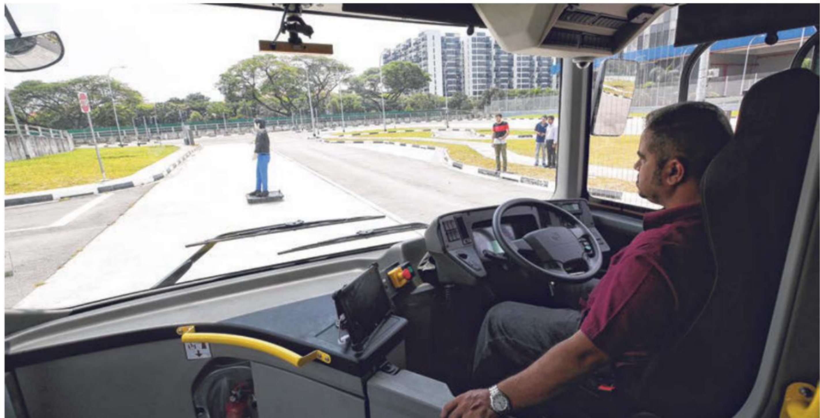
The NTU-LTA-Volvo Autonomous Bus (top left) running on a purpose-built track at Cetran. During a trial, the bus comes to a halt (above) when an errant “pedestrian” (represented by a moving dummy) is within sight. The bus is classified as having Level 4 autonomy – it can drive by itself but is still manned. ST PHOTOS: KEVIN LIM
