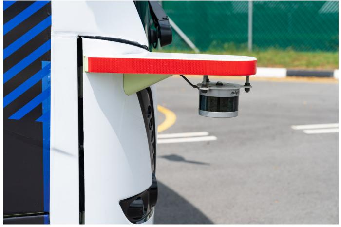
They include light detection and ranging sensors (LIDAR), plus stereo-vision cameras that capture imagery in 3D
