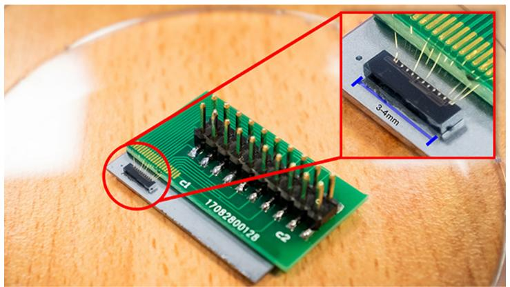
Roughly about 3mm in size, the tiny chip developed by NTU scientists uses quantum communication algorithms to better security than existing industry standards. It also opens doors for more secure communication technologies that can be deployed in compact devices such as smartphones, tablets and
