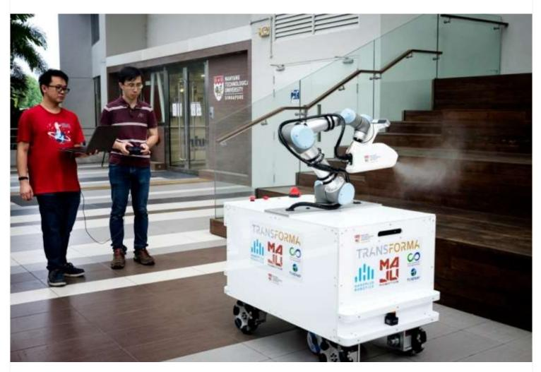
The XDBOT is controlled wirelessly and is semi-autonomous, removing the need for cleaners to be in contact with surfaces and reducing the risk of virus transmission (Image: NTU Singapore)
