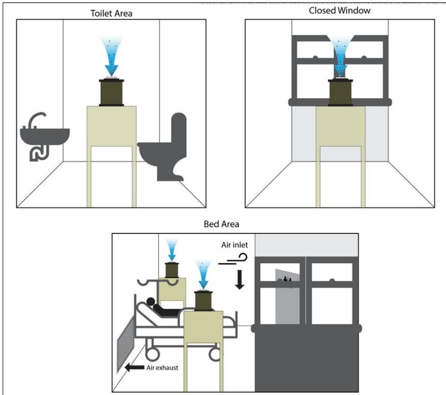
An infographic of how air sampling was done in a mechanically ventilated isolation ward.
