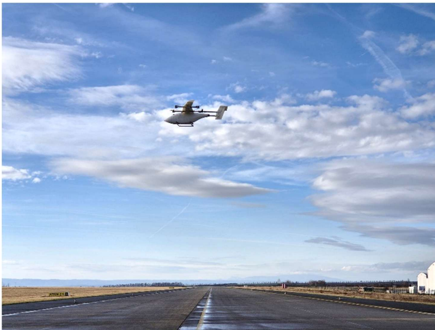
Photo 4 – The 3-metre wingspan prototype being flight tested in Germany in collaboration with the German Aerospace Centre DLR.
