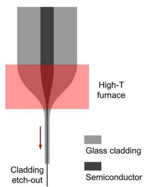
**Image:** A schematic diagram of the semiconductor fibre manufacturing method developed by the NTU research team.
