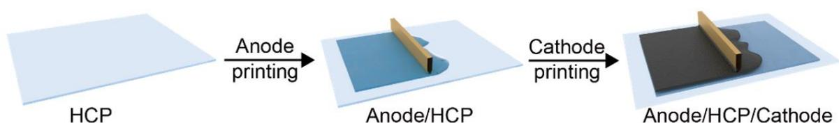
Image 1: Process of screen-printing the battery's electrode
