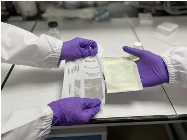
Image: The fabric-based energy harvesting prototype (right) developed by the NTU team contains a stretchable electrode (left) that is screen-printed with an ‘ink’ comprising a rubber-like material found in general purpose items such as teethers and handlebar grips.
