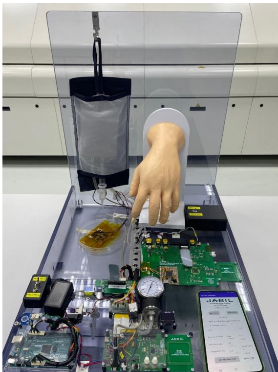
Image: Prototype of the JABIL-MTI Penang smart infusion system, which includes a low-cost intravenous (IV) fluid bag with an embedded printed sensor powered by
