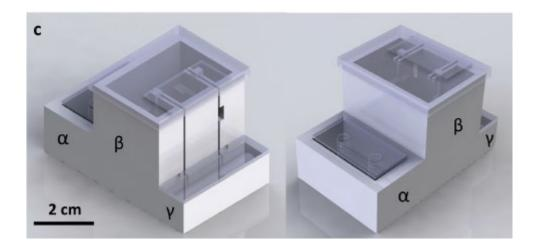
**Image 1:** The portable skin mapping device consists of three main parts ( $\alpha$ ) stamp sampling platform; ( $\beta$ ) skin patterning cell; and ( $\gamma$ ) power supply chamber/battery box.
