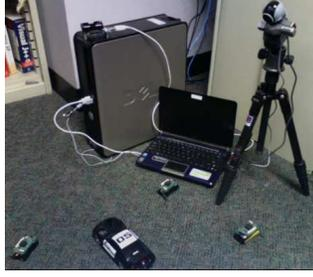
Figure 4. Testbed for acoustic target detection. 3 Iris motes and a webcam detect the moving toy car
