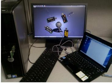
Figure 3. Testbed for light spot detection. 4 TelosB motes and a webcam detect the light spot.
