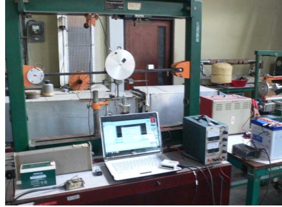
Fig. 1. Experimental set-up, which shows the simple vibration test rig, the Kyowa accelerometer mounted on the continuous beam, and other related instrumentations.
